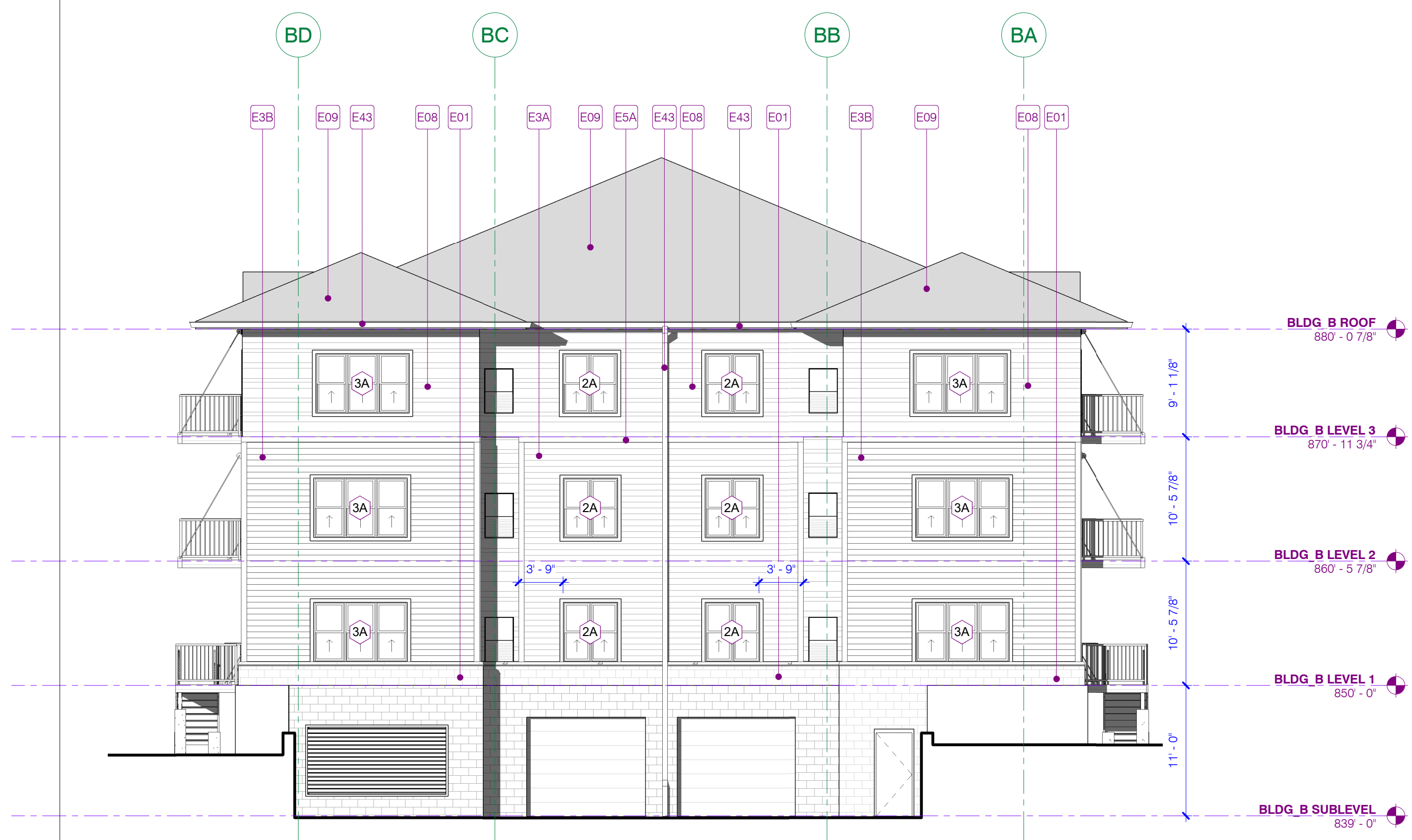
3 BLDG B - NORTH ELEVATION
